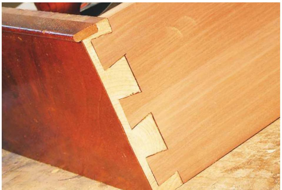
▲ Pic.13 The finished front-to-side drawer joint
